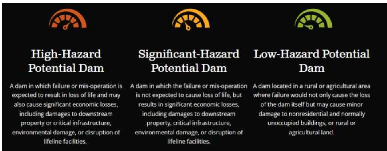
Figure 9-1. Dam Hazard Potential Classifications
